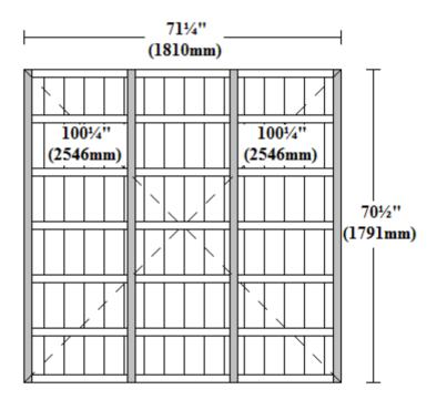
NB:- Floor joists run from left to right. Optional Floor Bearers run from front to back.
